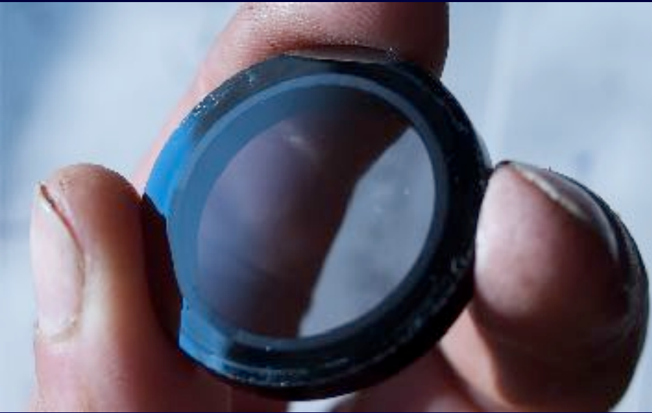
Pellicle Beam Splitter produced by National Photocolor Corp.
