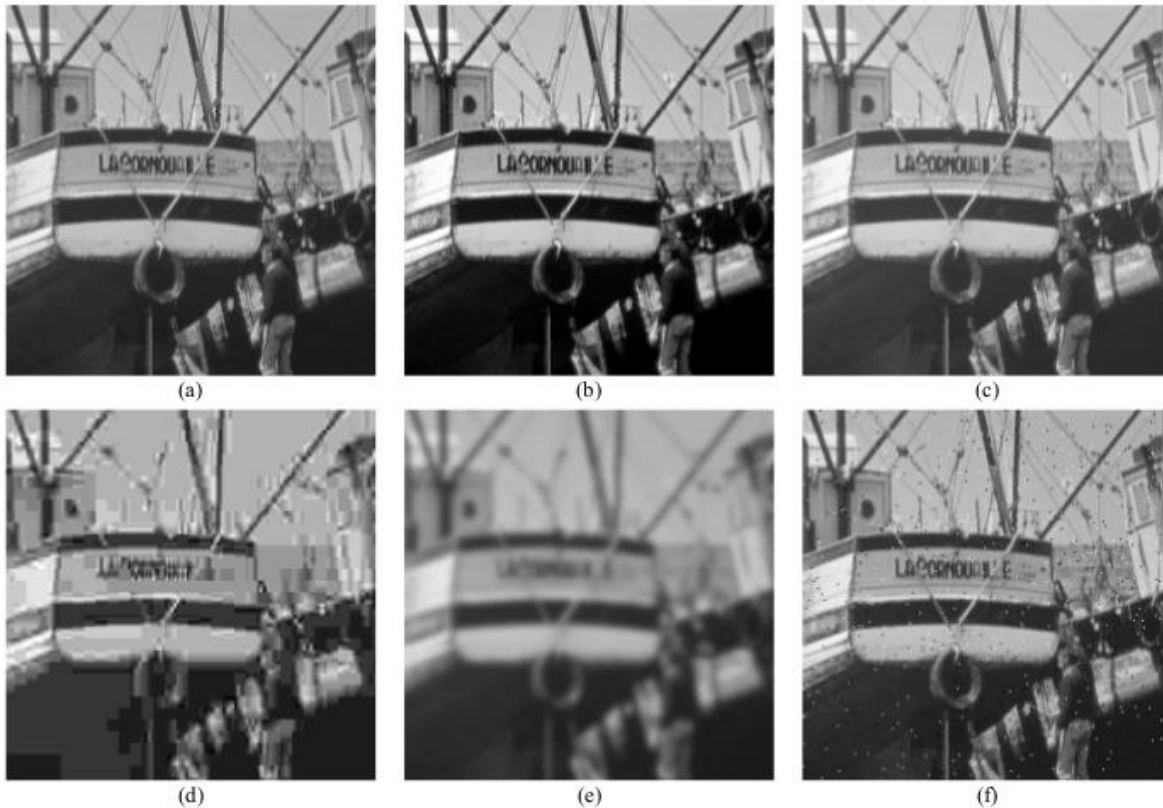
Fig. 2. Comparison of "Boat" images with different types of distortions, all with MSE = 210. (a) Original image (8bits/pixel; cropped from 512×512 to 256×256 for visibility); (b) Contrast stretched image, MSSIM = 0.9168; (c) Mean-shifted image, MSSIM = 0.9900; (d) JPEG compressed image, MSSIM = 0.6949; (e) Blurred image, MSSIM = 0.7052; (f) Salt-pepper impulsive noise contaminated image, MSSIM = 0.7748.
